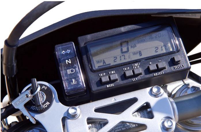
*\*The DR-Z400S's instrument panel has a tire circumference adjustment feature that allows you to fine tune the trip-meters for accuracy after mounting a knobby-style tire that may have a taller profile as compared to the original tire. This adjustment helps the dual tripmeter display be precise for the distance traveled so navigating using a roll-chart can be precise.*
