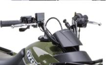
**Electric start system - with start-in-gear feature and recoil backup** – Start in gear system allows the engine to be started in any gear, when the left handlebar brake lever is pulled and the electric starter button is pressed. Low-maintenance precision electronic ignition system (CDI) is powered by a compact maintenance-free battery working with a 150 watt output charging system. DC power output for various electrical devices is optional.
