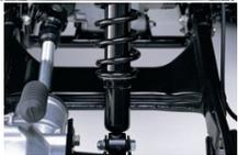
**Swingarm-type rear suspension** features single shock absorber with 5.5 inches of rear wheel travel, plus 8.3 inches of ground clearance for impressive performance over rough trails and terrain.
