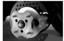
**Dual front hydraulic disc brakes feature pin-slide calipers and large 6.2-inch discs** feature large piston diameter and maximum brake pad surface area for increased stopping power and outstanding durability.
