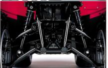
**Independent double-wishbone coil-over dual-shock absorbers front suspension** delivers 5.5 inches of wheel travel for a comfortable ride over all types of terrain.
