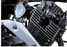
**Powerful full-size single-cylinder 246cc, SOHC, air-cooled 4-stroke engine** utilizing rubber engine mounts to reduce vibration and specific design features reduce mechanical noise for a quiet and comfortable ride. The cylinder is tilted 53° from horizontal for optimal air flow across the cooling surfaces of the cylinder head and cylinder. The engine is tuned broad powerband, with an emphasis on mid-range torque for impressive performance.
